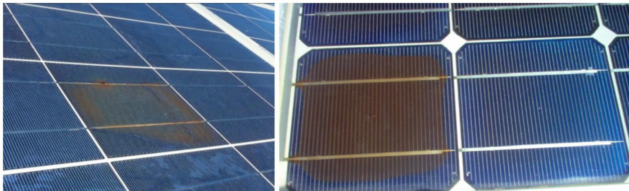
Figure 4 Left 10 year old polysilicon, Right 20 year old Monosilicon
